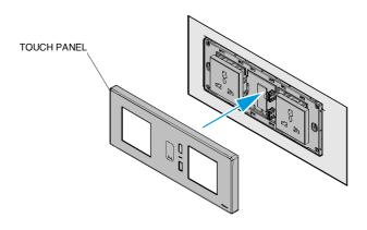
4. Carefully press the touch panel by applying even force on all sides until it is seated securely on the switch module.
